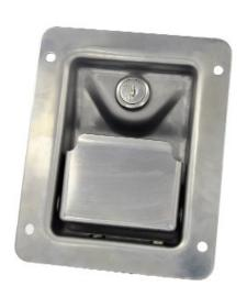
This compartment latch was designed for light to medium duty storage and compartment doors. Available in buffed stainless steel or plated mild steel, this product features a two point bellcrank for remote actuation and is power lockable.
